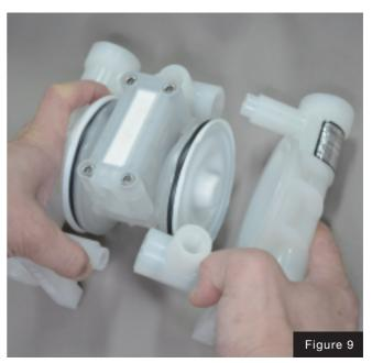
**STEP 9.** Remove liquid chambers by pulling chamber away from center section and inlet-discharge T-sections.
