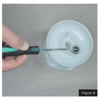
**STEP 6.** Remove the pilot spool retaining ring with an o-ring pick.
