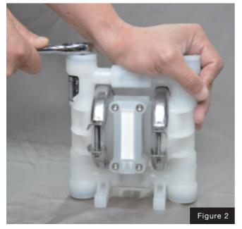
**STEP 2.** Use a ¼" socket wrench to remove the top retainer.
