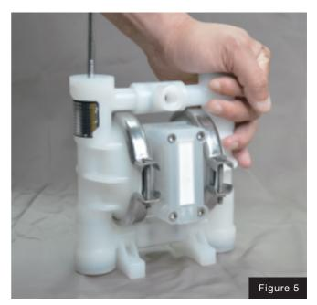
**STEP 5.** To remove valve seats, use approximately 3/16" rod or equivalent and push seats out from top to bottom.
