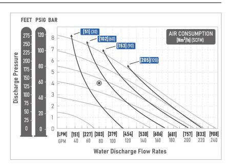
Flow rates indicated on chart were based on pumping water. For optimum life and performance, pumps should be specified so that daily operation parameters will fall in the center of the pump performance
