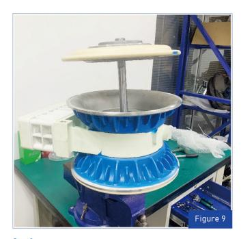
**Step 9.**Using an adjustable wrench, Rotating the diaphragm, and remove the diaphragm from the assembly.
