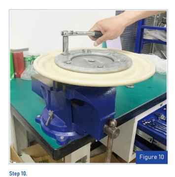
Remove the outer piston, diaphragm, inner piston from the assembly, replace with genuine Liquade parts for reliable performance.
