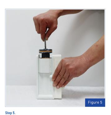
Remove air valve spool from air valve body by threading one air valve bolt into the end of the spool and gently sliding the spool out of the air valve body. Check the signs of the wear, replace the spool if necessary. The wear seals are not sold by separately.
