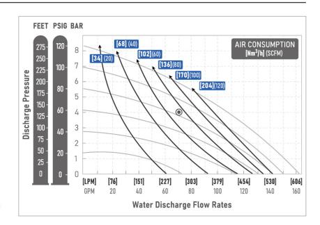
Flow rates indicated on chart were pumping water. For optimum life and performance, pumps should be specified so that daily operation parameters will fall in the center of the pump performance curve.
