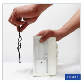
**Step 3.**Lift away air valve assembly and remove air valve gasket for inspection. Replace with Liquade gasket for reliable performance.
