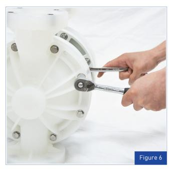
**Step 6.**Using a 9/16" wrench, remove the liquid chamber fasteners.
