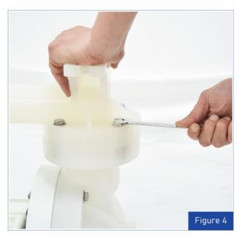
**Step 4.**Using a 9/16" wrench, loosen the discharge manifold from the liquid chambers.
