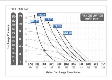
Flow rates indicated on chart were based on pumping water.
