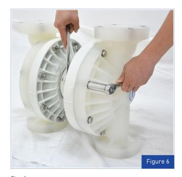
**Step 6.**Using a 3/4" wrench, remove the liquid chamber fasteners.
