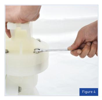
Step 4. Using a 3/4" wrench, loosen the discharge manifold from the liquid chambers.
