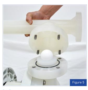
**Step 5.**Remove the inlet manifold, expose the valve balls, valve seats and 0 rings.
