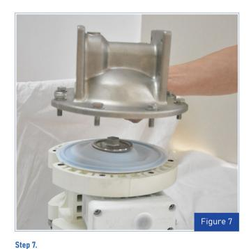
The liquid chamber should be removed to expose the diaphragm and outer piston. Rotate center section and remove the opposite liquid chamber.
