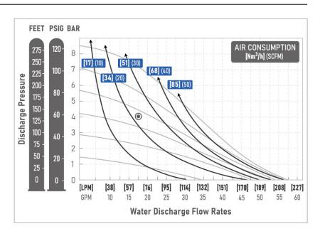
Flow rates indicated on chart were based on pumping water.
