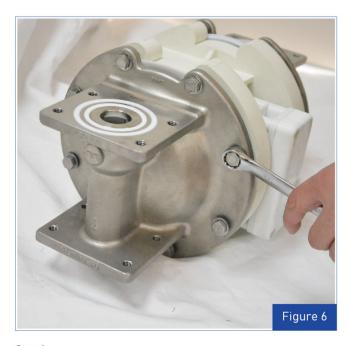
**Step 6.**Remove the liquid chambers from the center section with a 13 mm (1/2") box wrench.
