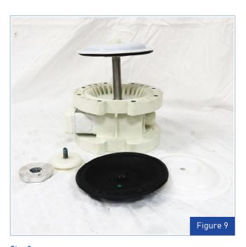
**Step 9.**Loosening and removing the outer piston, then assembly can be disassembled.
