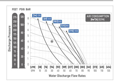
Flow rates indicated on chart were based on pumping water. For optimum life and performance, pumps should be specified so that daily operation parameters will fall in the center of the pump performance curve.
