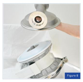
**Step 8.**Lift liquid chamber away from center section, check the diaphragm and outer piston.
