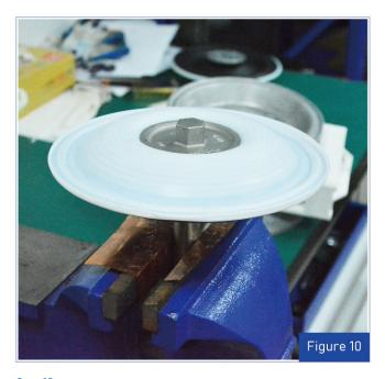
**Step 10.**Remove the outer piston, diaphragm, inner piston from the assembly, replace with genuine Liquade parts for reliable performance.
