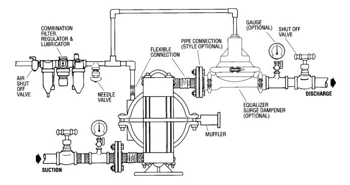
**NOTE:** In the event of a power failure, the shutoff valve should be closed, if the restarting of the pump is not desirable once power is regained.
