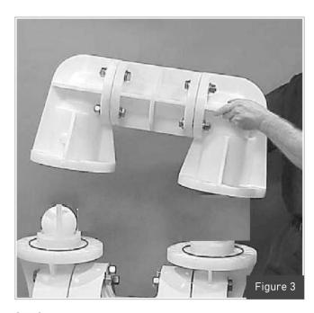
**Step 3.**Remove the discharge manifold, expose the valve balls, valve seats and 0 rings.
