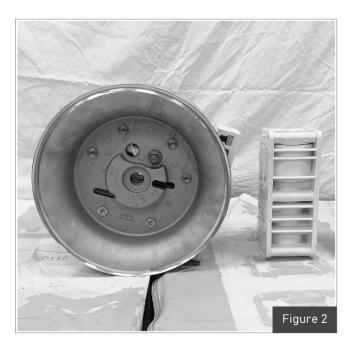
Step 2. Remove muffler plate and air valve bolts from air valve assembly, exposing muffler gasket for inspection. Replace with Liquade gasket for reliable performance.
